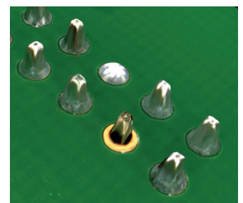
Insufficient wetting (front) and missing pin (back)
